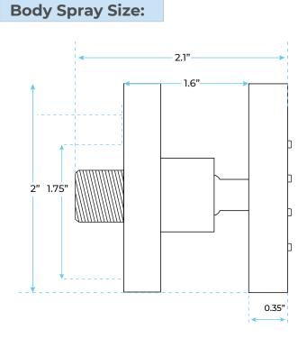
Thread Interface Size: G 1/2 Inch Function: Rainfall Shower Head Feature: Water Saving Shower Heads Type: Fixed Rotatable Type Installation Type: Wall Mounted
